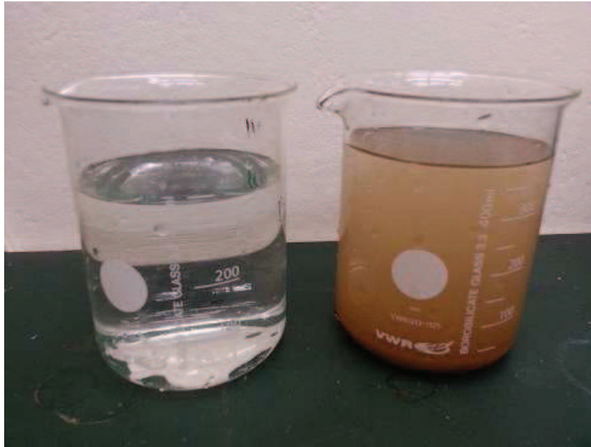
Figure 4.6: Water samples. On the left permeate sample and on the right sMBR tank sample
