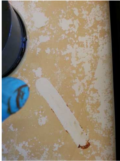
Figure 4.9: Fouling onto membrane surface.
