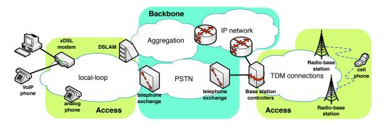
Figure 2.15: Access and backbone portions of a network
