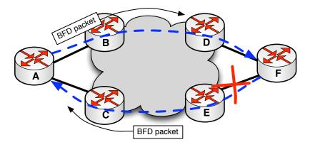
Figure 2.27: End-to-end failure detection mechanisms
