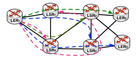
Figure 2.24: IP/MPLS tunnels with traffic engineering
