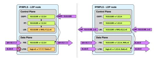
Figure 2.23: LDP incremental assignment of labels
