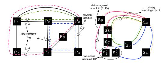
Figure 1.7: Example deployment of SDH/SONET rings
