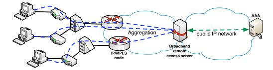
Figure 2.16: Aggregation and public portions of a backbone
