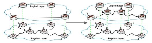
Figure 3.6: Non-disjoint lightpaths implementation and an alternate configuration.
