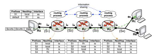
Figure 2.17: Forwarding and routing processes
