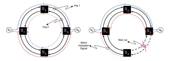
Figure 1.5: Transmission over rings and SNCP/UPSR (1+1) implementation
