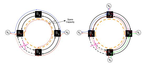
Figure 1.6: Protection based on MS/BLSR (1:1 and 1:N)
