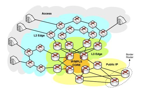
Figure 5.25: Scheme of ANTEL's convergent levels
