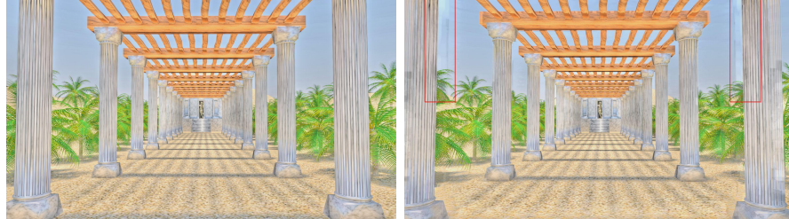
Figure 3.14: Ghosting Artifacts appearing on two successive frames. It is most noticeable around the two forefront columns (red squares).
