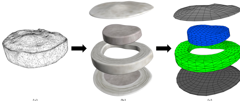
FIGURE 3.5 – The four component of the structure of inter-vertebral discs : the two endplates, the annulus and the nucleus. (a) : surface mesh from [MFT*09]. (b) : Our textured mesh. (c) : Our volumetric mesh.
