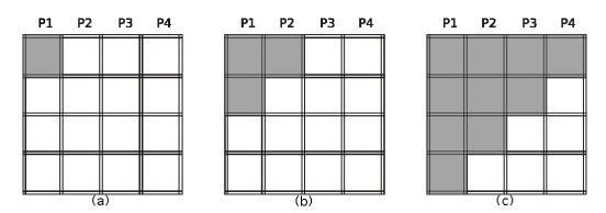
Figure 4.4: The wavefront method.
