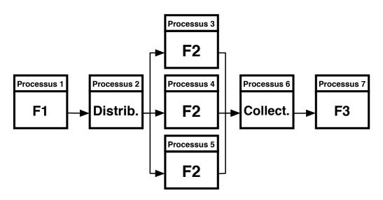
Figure 2.3: A sample process graph
