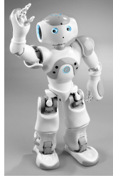
Figure 7.11: The Nao robot. A single degree of freedom is considered in the experiments, the angle of the arm.
