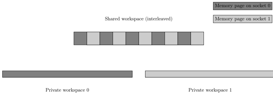
Figure 3.2: Illustration of the adaptation of the ALGTIME factorization phase for NUMA architectures on an example with two threads under \mathcal{L}_{th} , each mapped on a core of different sockets, and both working together above \mathcal{L}_{th} .
