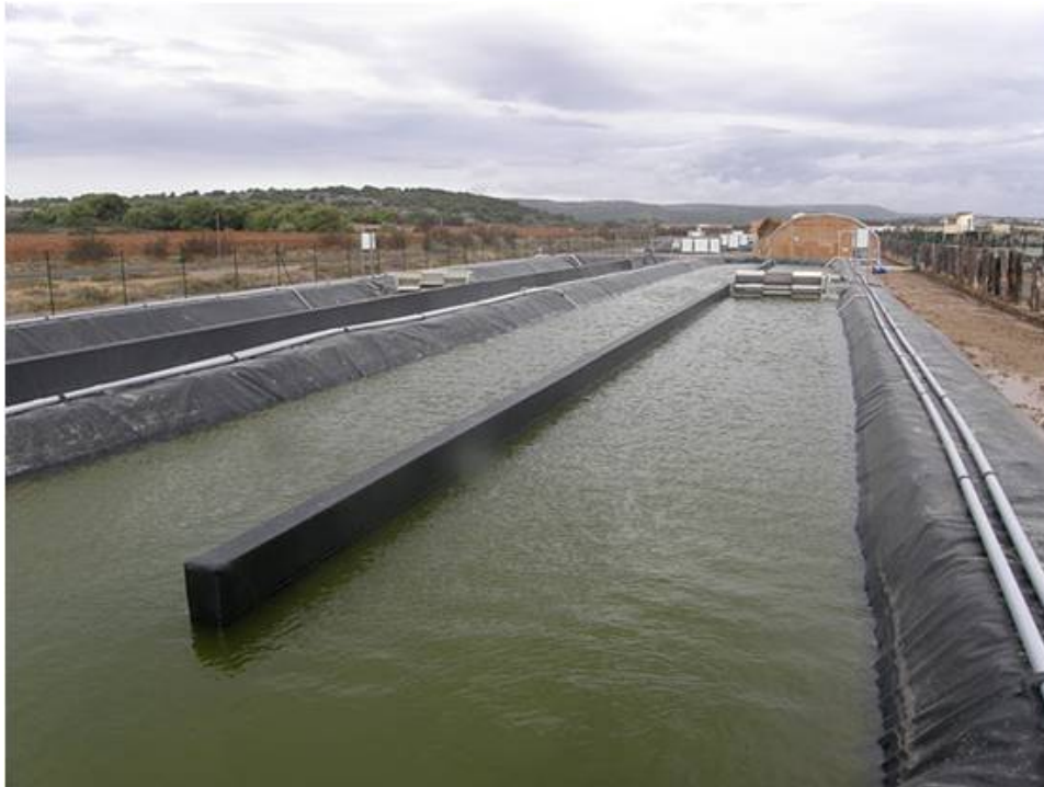
Figure 1: Industry-Scale raceway culturing system (project salinalgue)
