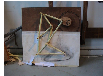
(d) Actual leg are based on basic plastic rods.
