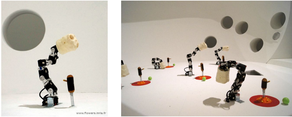
Fig. 7.2.: Ergo-robot are a 6 DoF serial robots with a stem shape those were developed in the Flowers Lab. In particular, they were involved for the Fondation Cartier exhibition (see chapter 10)
