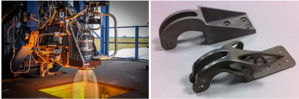
(a) The SuperDraco rocket engine has a combustion chamber: 3D-printed - SpaceX. (b) A conventional hinge is seen in the background and a 3D-printed metal hinge is seen in the foreground - EADS.
