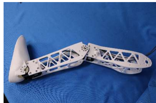
(b) Poppy's leg mechanical structure
