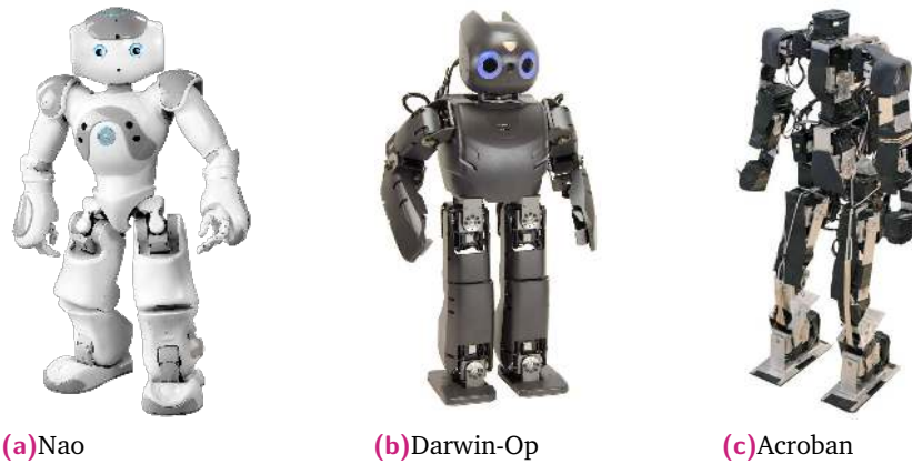
Fig. 6.1.: None of the existing platforms in 2012 were suitable for exploring the role of morphology. Nao was impossible to modify. Darwin Op and Acroban used aluminium parts that are really difficult and expensive to produce.
