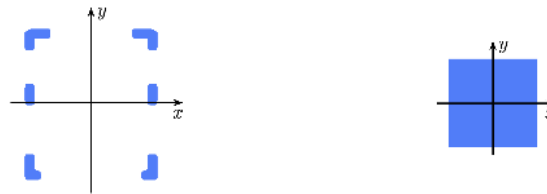
Fig. 6.7.: Comparison of poppy's leg section and a rectangular beam having the same second moment of area.
