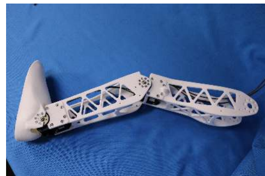
(b) Poppy's leg mechanical structure
