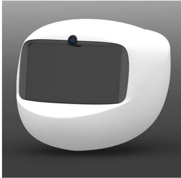
Fig. 6.24.: A preview of the new design for Poppy's head. As we want to show expressive eyes on the screen, we have replaced the two cameras with big lenses of Poppy beta by a small one, thus cameras are not misunderstood as Poppy's "eyes".
