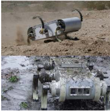
(a) The Rhex robot is a compliant hexapod able to move quickly and robustly over complex terrain.
