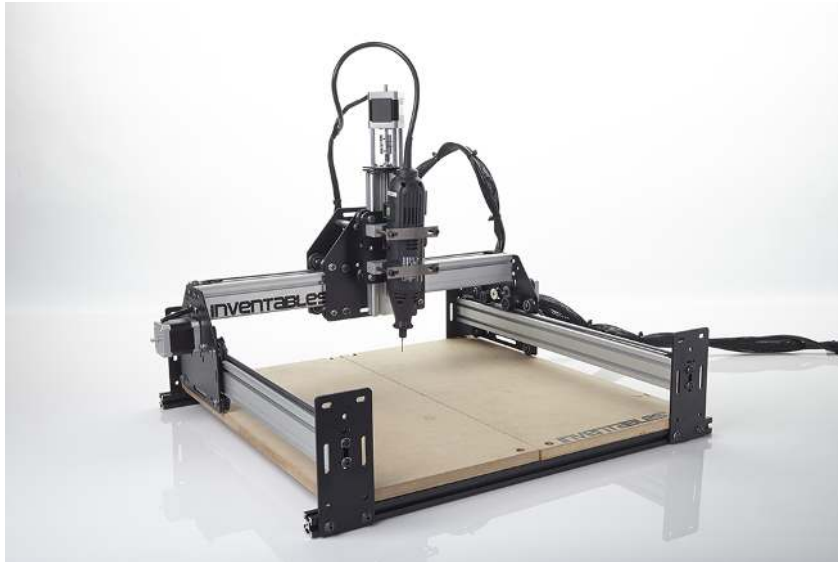
Fig. 4.12.: The shapeoko v2 is a low cost and open source CNC 2.5 axes.
