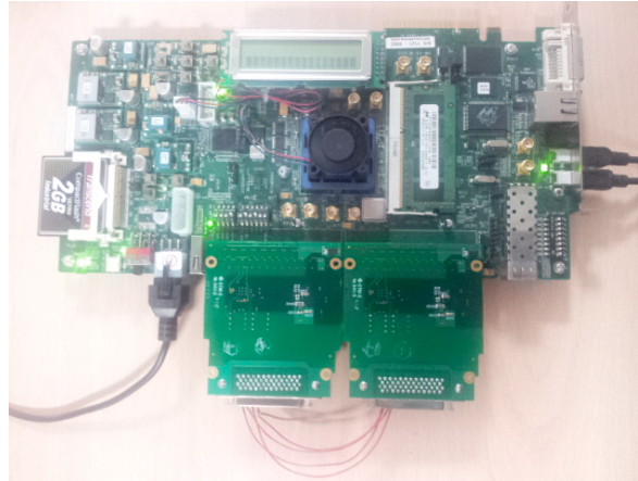
FIGURE 2.16 – ML605 kit showing FMC connector loopback using MIL-STD-1553
