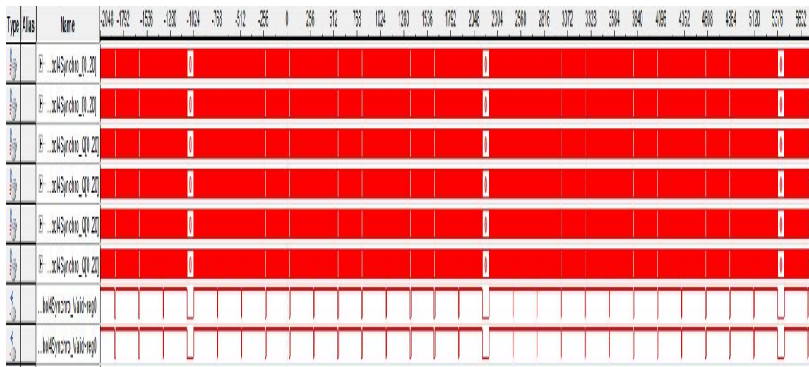
FIGURE 5.18: Altera SignalTap Snapshot of coarse synchronization output. Presence of periodic zeros indicate cyclic prefix removal and bigger gap zeros indicate the removal of the first training symbol in the output fed into FFT block.
