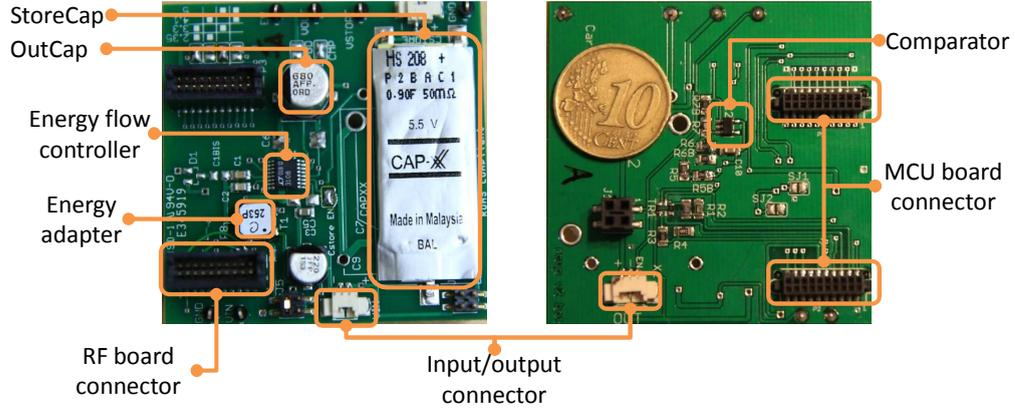
FIGURE 2.9: Hardware design of MESC.
