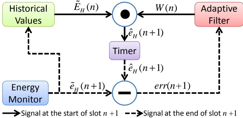
FIGURE 3.6: Energy predictor using adaptive filter architecture. Historical harvested energy profile is kept in a vector  $\tilde{E}_H(n)$  to predict  $\hat{e}_H(n+1)$  at the beginning of slot  $(n+1)$ . Until the end of slot  $(n+1)$ ,  $\tilde{E}_H(n)$  and  $W(n)$  are updated from  $err(n+1)$ .
