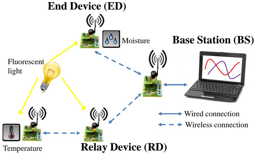
FIGURE 5.1: Multi-hop energy harvesting wireless sensor network.
