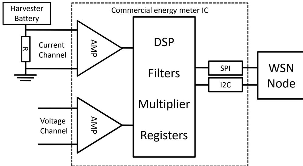
FIGURE 3.2: Generic architecture of a hardware-based energy monitor.
