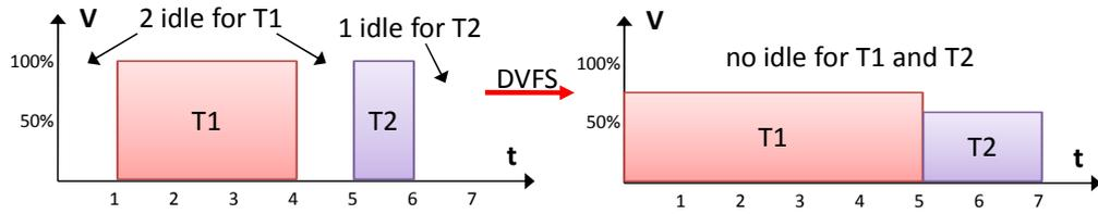
FIGURE 1.4: Two tasks are scaled by using DVFS technique.
