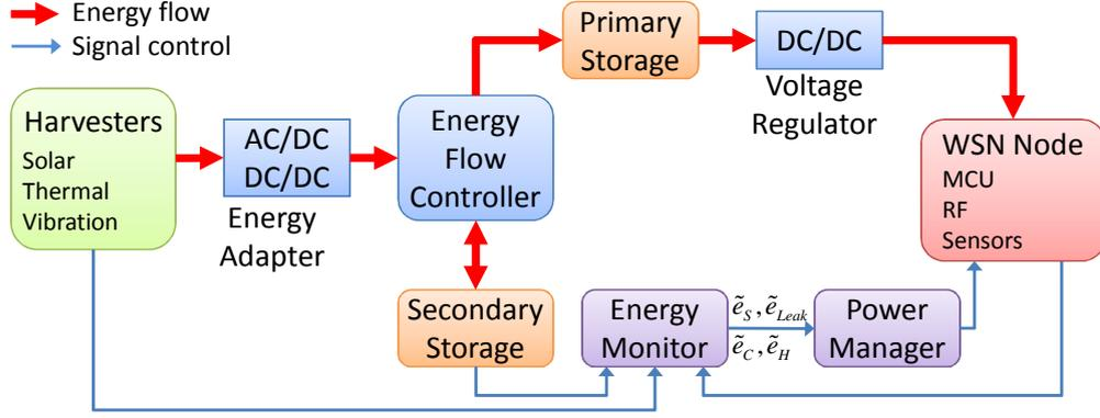
FIGURE 3.1: Energy monitor in the dual-path architecture.
