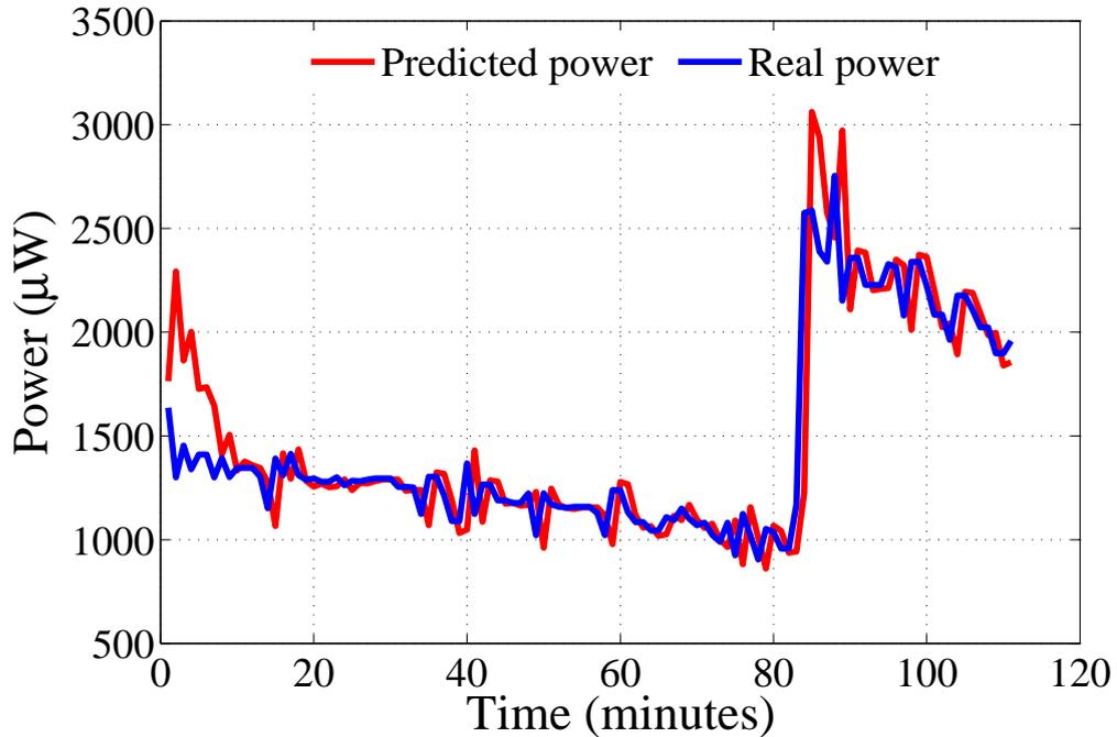
FIGURE 3.10: Energy prediction of harvested energy recorded by a PowWow node near a window in an office with  $p = 1$  and  $\mu = 0.3$ . At around 80 minutes, the curtain is opened and the harvested power suddenly increases.
