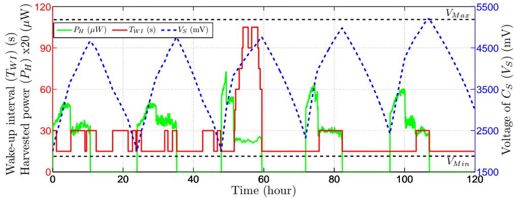
FIGURE 5.16: Adaptations of ED(1) using WVR-PM with  $\Delta = 15$ .
