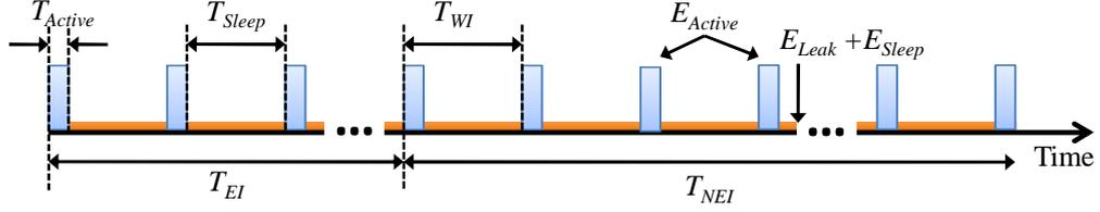
FIGURE 2.10: Communication of the WSN node during a cycle of the periodic source including the harvesting and non-harvesting energy interval ( $T_{EI}$  and  $T_{NEI}$ ). However, the harvested energy is only available during  $T_{EI}$ .
