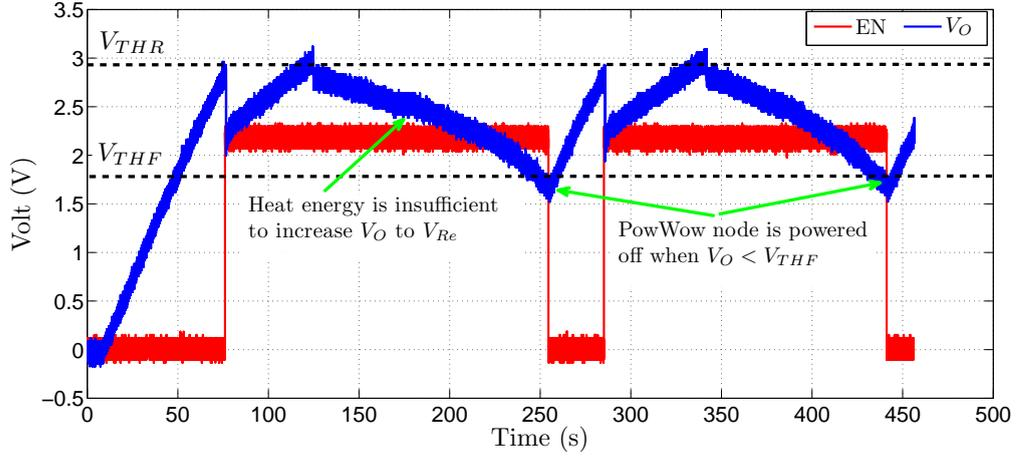
FIGURE 2.13:  $V_O$  with thermal energy. After initializing the RF transceiver, the thermal energy is only enough to charge  $V_O$  to  $V_{Re}$ . More harvested power is required to satisfy ENO of EH-WSN node.
