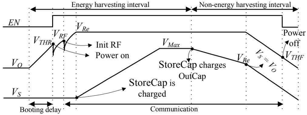
FIGURE 2.8: System operation diagram of MESC (time and voltage are not scaled). During the harvesting energy interval, the WSN node is kept shut down until  $V_O$  reaches  $V_{THR}$ . During the non-harvesting energy interval, the WSN node is turned off when  $V_O$  decreases below  $V_{THF}$ .
