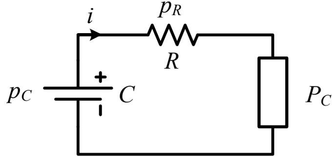
FIGURE 3.4: Generic model for the supercapacitor.
