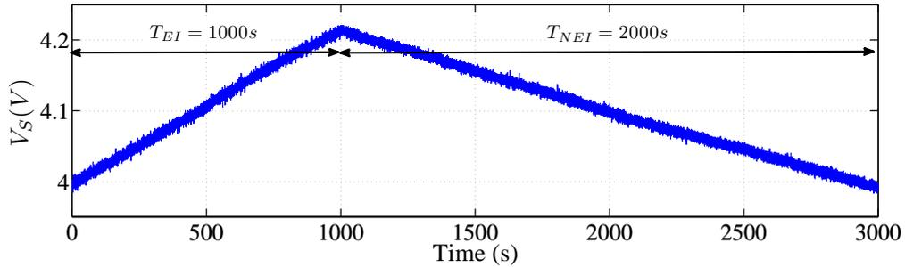
FIGURE 2.14:  $V_S$  of a PowWow node powered by two PVs when  $T_{WI} = 52s$ . The harvested energy buffered during  $T_{EI} = 1000s$  is used in the next 2000s when the environmental energy is no more available ( $T_{NEI}$ ).
