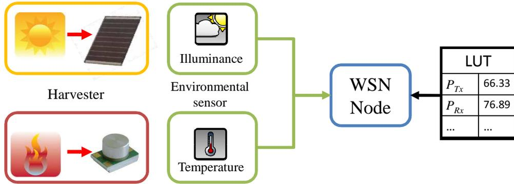
FIGURE 3.3: Generic architecture of a software-based energy monitor.
