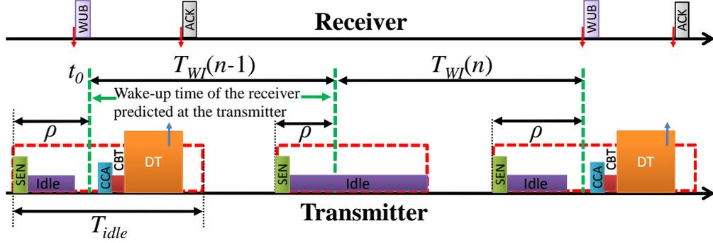
FIGURE 5.6: Synchronized wake-up interval MAC protocol for low wake-up variations multi-hop EH-WSNs (SyWiM).
