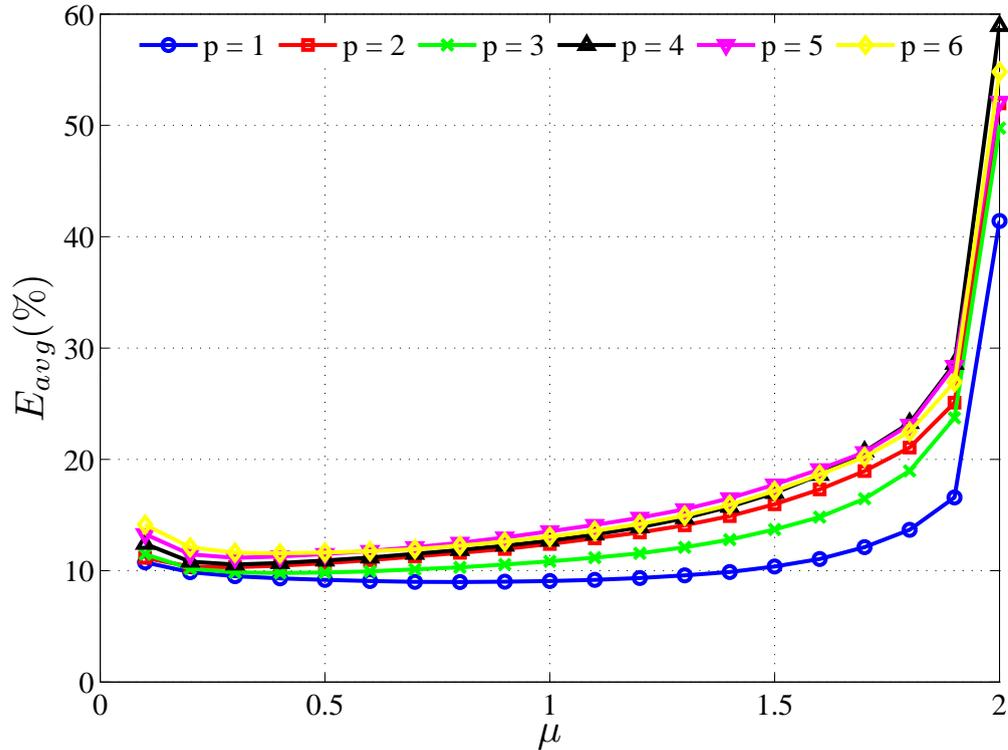
FIGURE 3.9: Average error of the energy predictor when applied to wind energy in seven consecutive days. With the same order and step size as solar prediction ( $p = 1$  and  $\mu = 0.3$ ), the average error is 9.1%.
