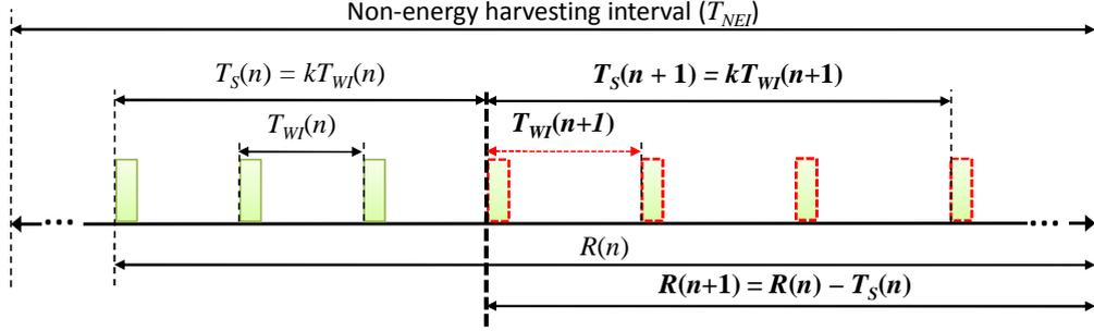
FIGURE 5.4: Negative energy power manager (NE-PM) for non energy harvesting interval ( $T_{NEI}$ ). The next wake-up interval ( $T_{WI}(n+1)$ ) is estimated from the remaining duration of non energy harvesting and current energy in StoreCap.
