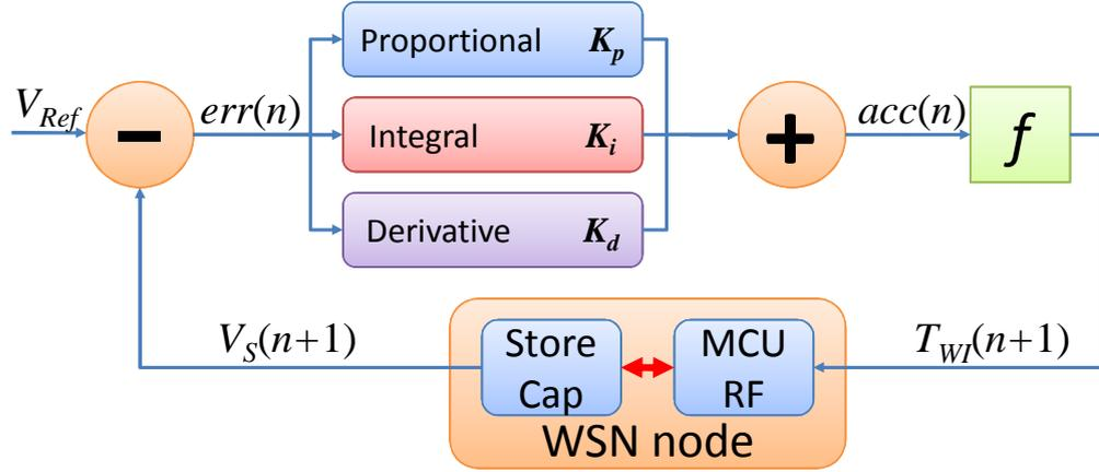
FIGURE 4.3: PID controller-based power manager (PID-PM) with three components: Proportional, Integral and Derivative. Adaptive function  $f$  updates the next wake-up interval of the WSN node ( $T_{WI}(n+1)$ ) according to accumulated error  $acc(n)$ .
