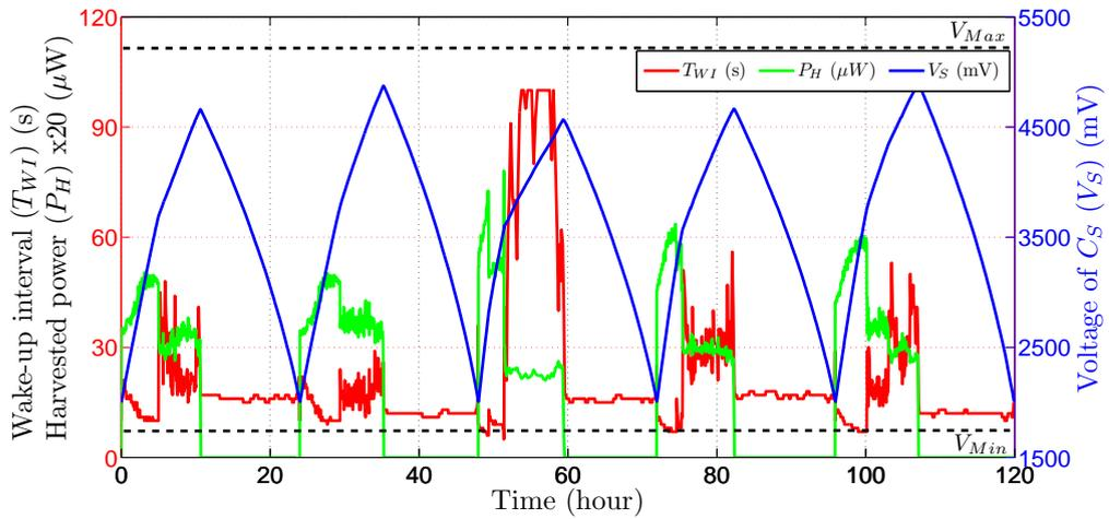
FIGURE 5.12: Adaptations of ED(1) using WVR-PM with  $\alpha_C = 0.9$ ,  $\alpha_H = 0$  and  $\Delta = 1$ . The variation of  $T_{WI}$  is significantly reduced during  $T_{NEI}$  as  $\hat{e}_{Active}(n+1)$  is very close to  $\hat{e}_{Active}(n)$  when  $\alpha_C = 0.9$ . Over five days, the variation is reduced down to 60% in average.TABLE 5.5: Average  $Nb\_Var$  and  $Sum\_Var$  and their gain compared to PEO-PM ( $\alpha_C = 0.5$ ) over five days ( $\alpha_H = 0$ ,  $\Delta = 1$ ).
