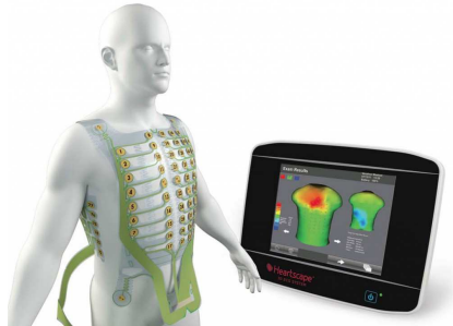
Figure 2.9: Vest used for the ECGI method. From arwatch.co.uk
