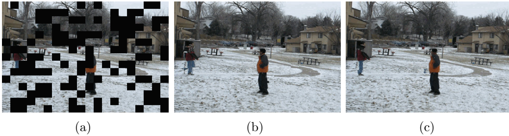
Figure 3.15: Performances of the proposed approach in the error concealment application. Sequence Duo. (a) Image with 50% of 16 \times 16 blocks are lost (first column), PSNR= 9.01 dB. (b) Image recovered using motion compensation (second column), PSNR= 28.26 dB. (c) Image recovered using the proposed algorithm (third column), PSNR= 32.23 dB.
