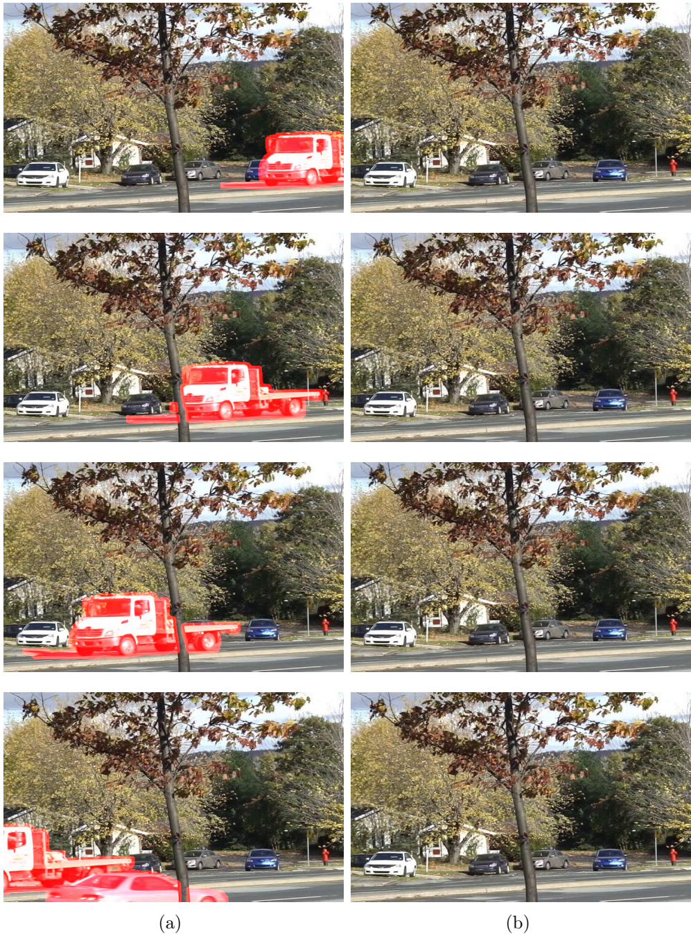
Figure 5.9: Inpainted results of change detection video sequence with dynamic background: fall(720 × 480). Sequence with large hole. (a) Input image with the mask of object to be removed. (b) Inpainted result using the proposed approach.
