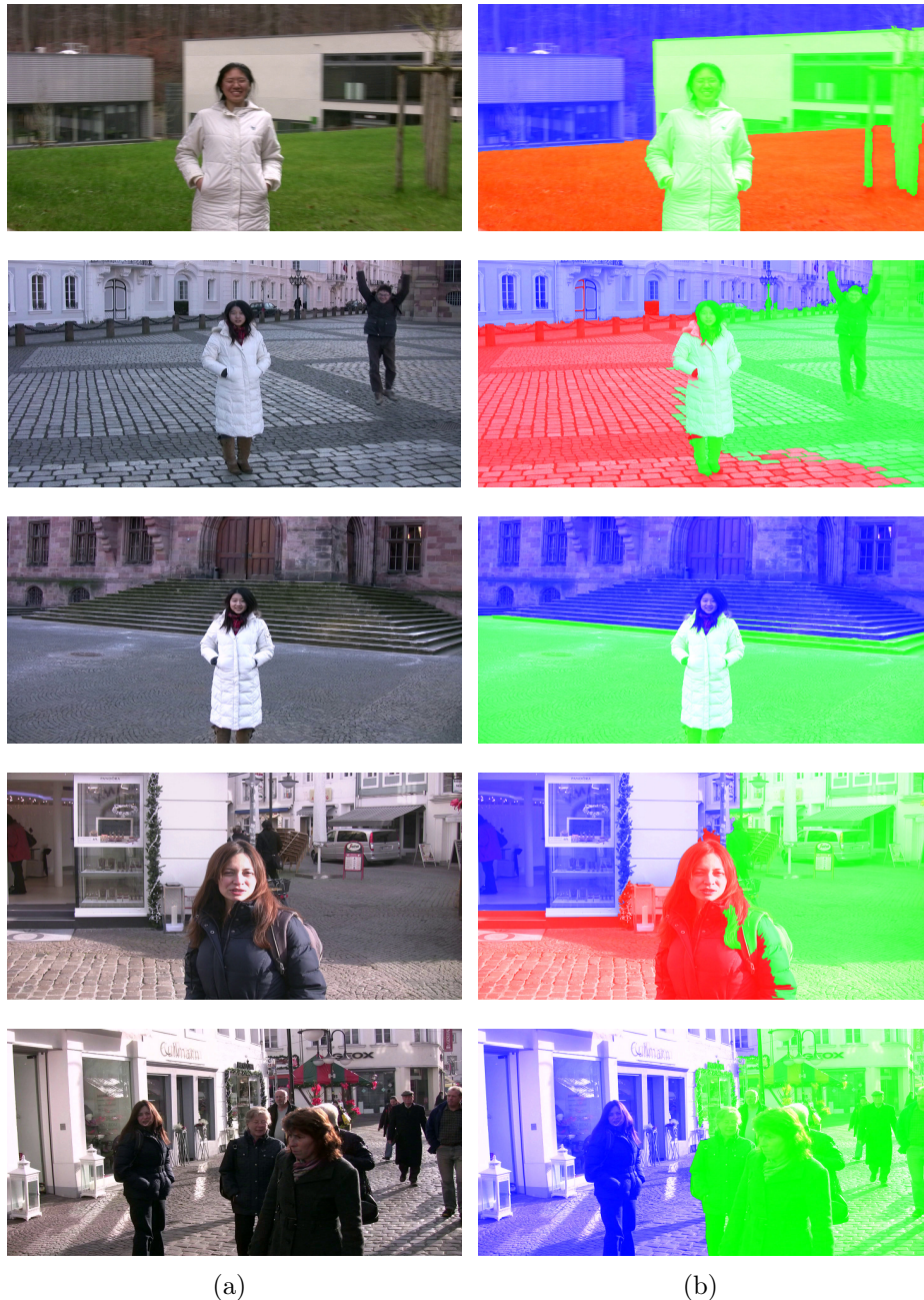
Figure 6.11: Samples of region segmentation results using Mean Shift [119]. (a) Original images. (b) Images with segmented regions.
