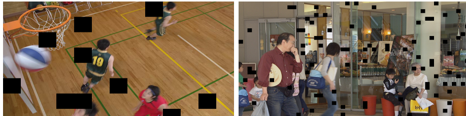
Figure 3.16: Test video sequences: BasketBallDrill and BQMall of resolution 832 \times 480 and the frame rate is 50 fps with a loss rate of 5% and blocks of sizes 64 \times 64 and 16 \times 16 .
