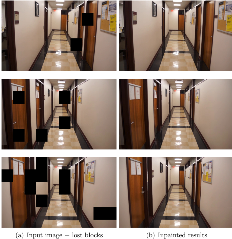
Figure 6.18: Test frames from Scene12 video sequences with varying lost rate. From top to bottom 5%, 10% and 20% of the 64 \times 64 blocks are lost.
