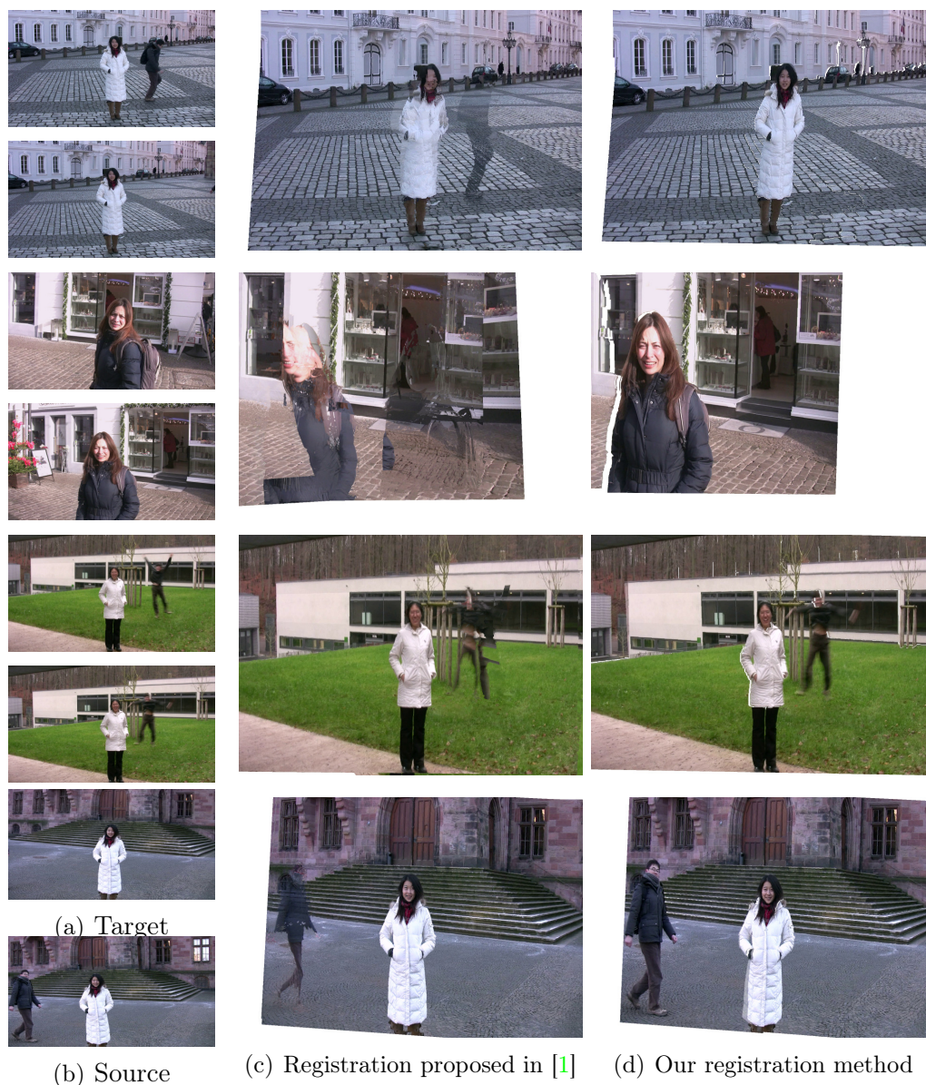
Figure 6.12: Comparison of registration quality with scenes having different types of camera motion. First row: slow rotation. Second row: fast view changes. Rows 3 and 4: small view change and zooming. (a) Target image. (b) Source image(to be registered to the target). (c) Registration result using our implementation of registration approach proposed in [1]. (d) Registration result using our proposed registration approach.
