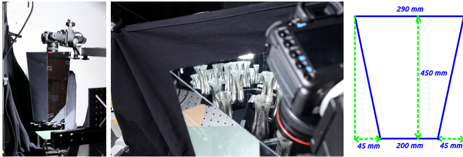
Figure 5.5: Photograph of our practical setup, left. A view inside showing the mirror space, middle. Draft of one of the three identical mirrors in the kaleidoscope, right.
