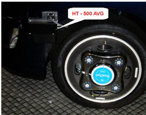
Figure 7.4: Laser sensor for chassis height measurement
