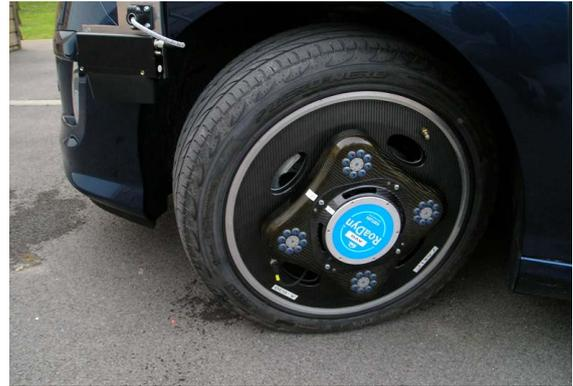
Figure 7.3: Kistler wheel force transducers at front left wheel
