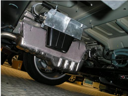
Figure 7.2: The Correvit installed at place of the spare wheel
