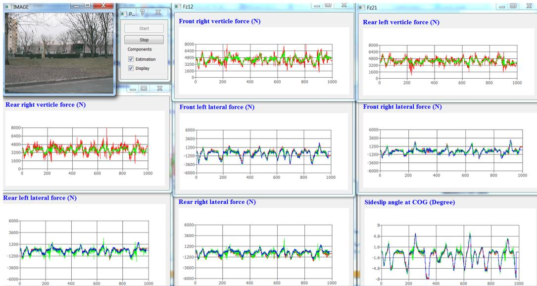
Figure 7.12: Onboard real-time estimation surveillance interface
