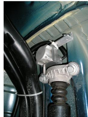
Figure 7.5: Suspension deflection sensor
