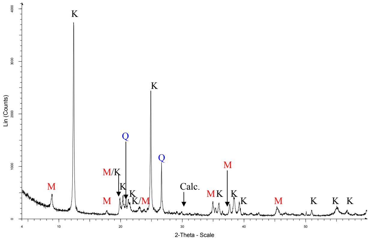
Figure II- 4 : Diffractogramme de la kaolinite Polwhite. M = Muscovite, K = Kalonite, Q = Quartz, Calc. = Calcite
