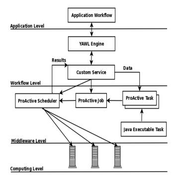
Fig. 10. Interaction Between ProActive and YAWL
