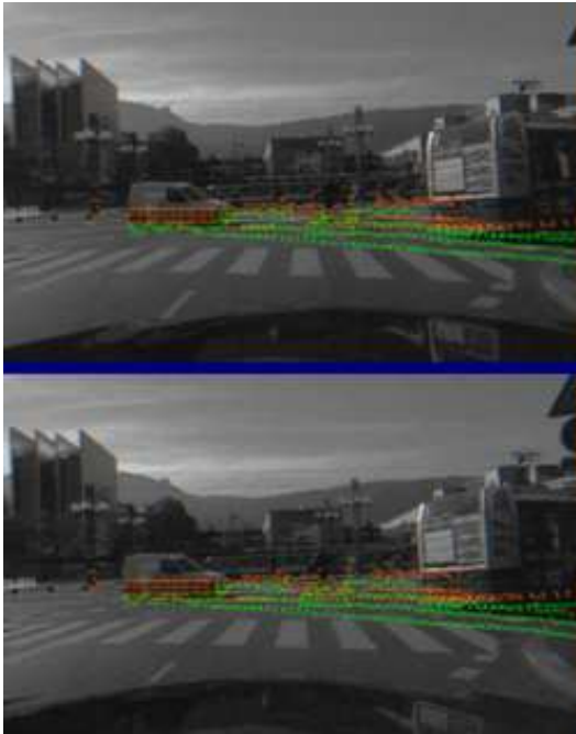
Fig. 5. An example of the multi-layer telemetric data represented by laser impacts (colored dots) from the two on-board lidars
