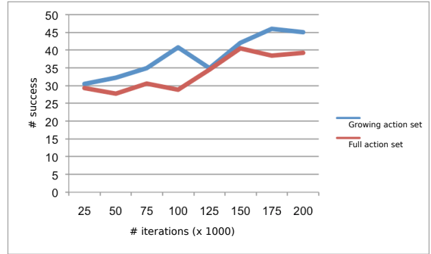
Fig. 5. Using configuration (1). Directly learning with the full set of actions is less efficient than learning with only 3 actions and, then (around iteration 100.000) using 5 actions. This results comes from only one experiment with the robot, as policy evaluation, done every 25.000 iteration, takes about 20 minutes.
