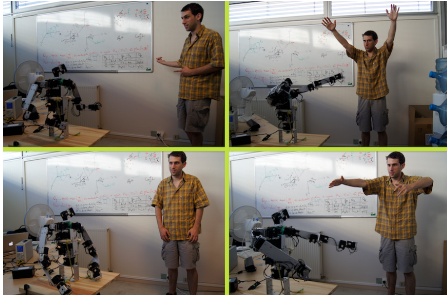
Figure 6: The robot arms are in the same position than the user's ones
