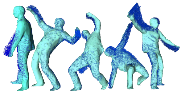
Figure 1: Example of dense scene flow (in blue) from sparse 2D and 3D features and dense normal flow constraints (as for the rest of the paper, figures are best viewed in color).
