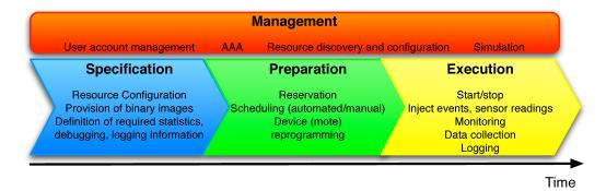
Fig. 4. Experiment execution workflow and corresponding testbed services.
