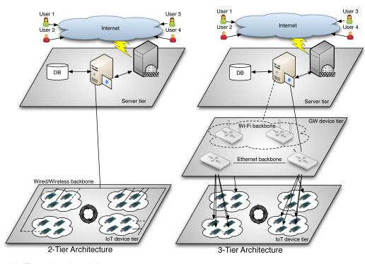
Fig. 2. Typical IoT testbed architectures.
