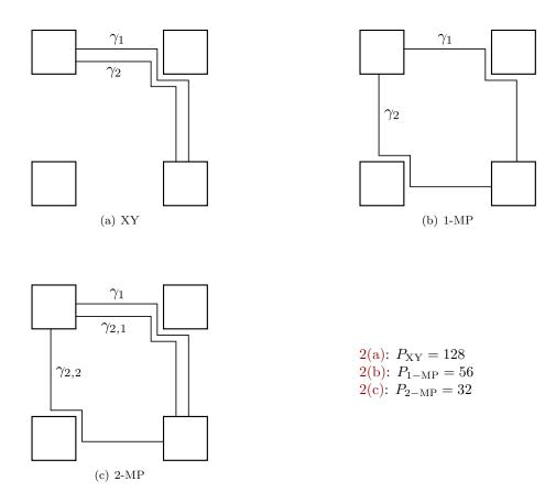
Figure 2: Comparison of routing rules.
