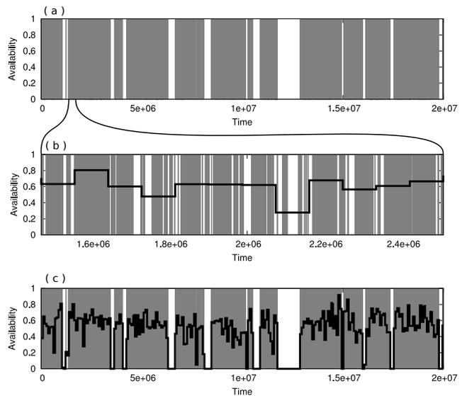
**Figure 1:** The gray areas represent resource availability, the black line represent a one-day integration: (a) eight months of raw traces; (b) twelve-day zoom with raw and integrated traces and (c) same as the first plot, plus one-day integration.
