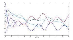
Fig. 2. States (solid line) and their (dashed line) estimation with a HOSMD
