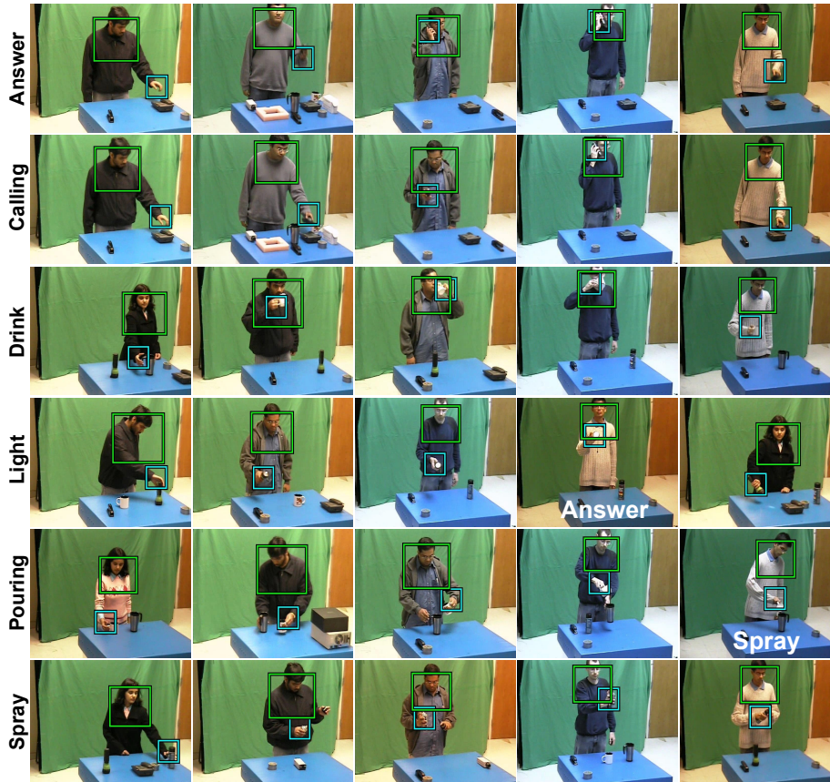
Figure 11: Human-object pairs localized on the Gupta video test set with the combined classifier. Each row shows one frame of the five test sequences of a class. Actions in this dataset follow precise motion patterns: each row displays samples selected to follow the temporal pattern. The two only misclassified samples are indicated with the incorrect class label overlaid.
