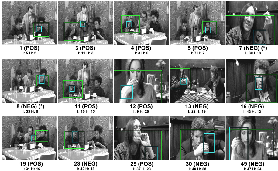
Figure 10: Smoking results. Human-object pairs localized in test videos. The ordering corresponds to the ranking of the combined action classifier. We also show the rank of the individual classifiers ( I : interaction classifier, H : 3DHOG-track classifier). In many cases the interaction and 3DHOG-track classifiers agree and assign both a high score to a positive sample. Complementary scores are obtained for samples 16, 23, 30 and 49: the interaction classifier correctly penalizes these negative samples without correct object motion, whereas 3DHOG-track is unable to distinguish them and assigns high scores. Note that sample 49 is a true negative, as it represents a person holding a cigarette and not smoking. For sample 19 the object track does not cover the correct object, thus the interaction classifier gives a low score, whereas the 3DHOG-track classifier assigns a high score. (*) For the smoking action we point out that the imprecise temporal extent of the annotations sometimes leads to an incorrect evaluation: samples 7 and 8 show a person smoking, but do not meet the spatio-temporal overlap threshold with the annotations.
