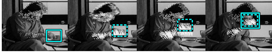
Figure 4: The LDOF-MS tracker at test time. In the first frame (left) the cup is automatically detected by an object detector. In the subsequent frames no detections are found on the cup. LDOF-MS produces an object track (dashed window) by propagating the detection from the first frame according to point tracks (white segments). In the last frame (right) the cup is again detected. LDOF-MS adds this detection to the track and uses it to update the confidence score, but not the location of the track.
