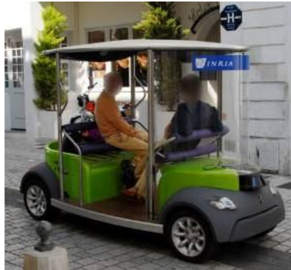
Fig. 3. Yamaha AGV by INRIA: CyBus vehicle
