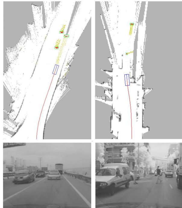
Fig. 3. Mapping and moving objects detection results. A bicycle and an oncoming moving car have been successfully detected.
