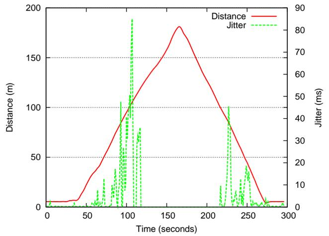
Figure 7: UDP range test with 2 cars (dist./jitter).
