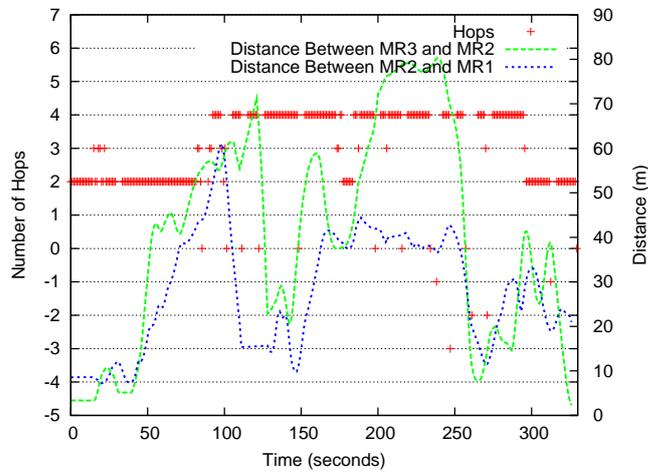
Figure 16: Ping highway test with 3 dynamic cars (hops/dist.).
