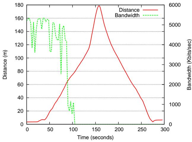
Figure 8: TCP range test with 2 cars (dist./band.).
