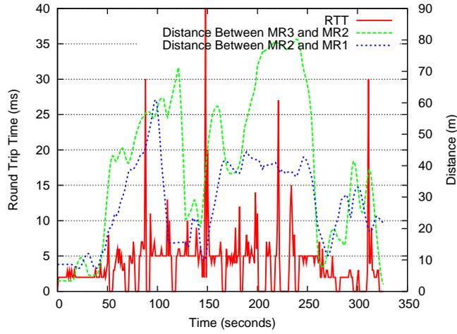
Figure 15: Ping highway test with 3 dynamic cars (RTT/dist.).
