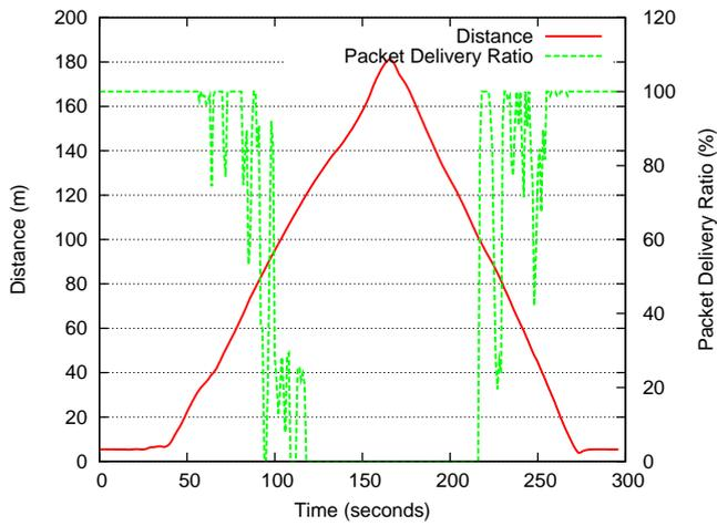
Figure 6: UDP range test with 2 cars (dist./PDR).
