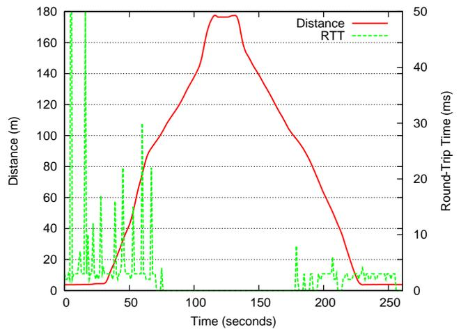
Figure 9: Ping range test with 2 cars (dist./RTT).
