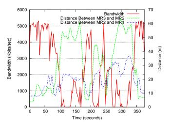
Figure 14: TCP highway test with 3 dynamic cars (band./dist.).
