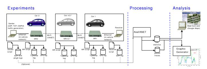
Figure 2: System overview and data processing units.
