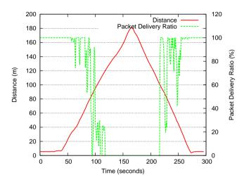
Figure 6: UDP range test with 2 cars (dist./PDR).
