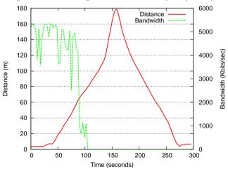
Figure 8: TCP range test with 2 cars (dist./band.).
