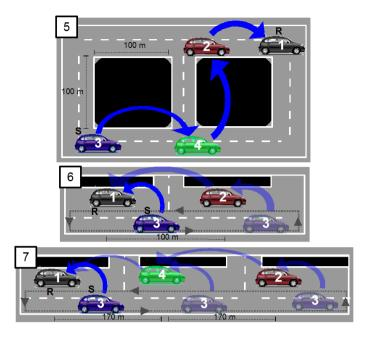
Figure 4: Overtaking and four-vehicles tests.
