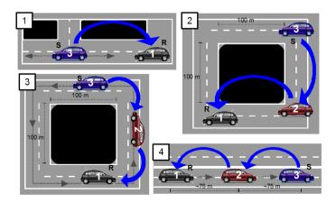
Figure 3: Maximum range and three-vehicles tests.
