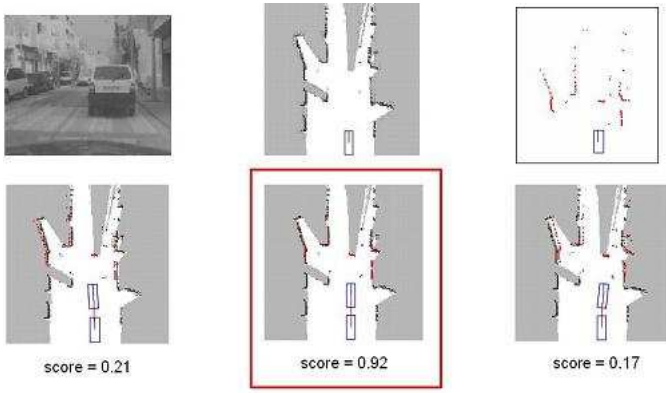
Fig. 3. An example of localization on the Daimler demonstrator
