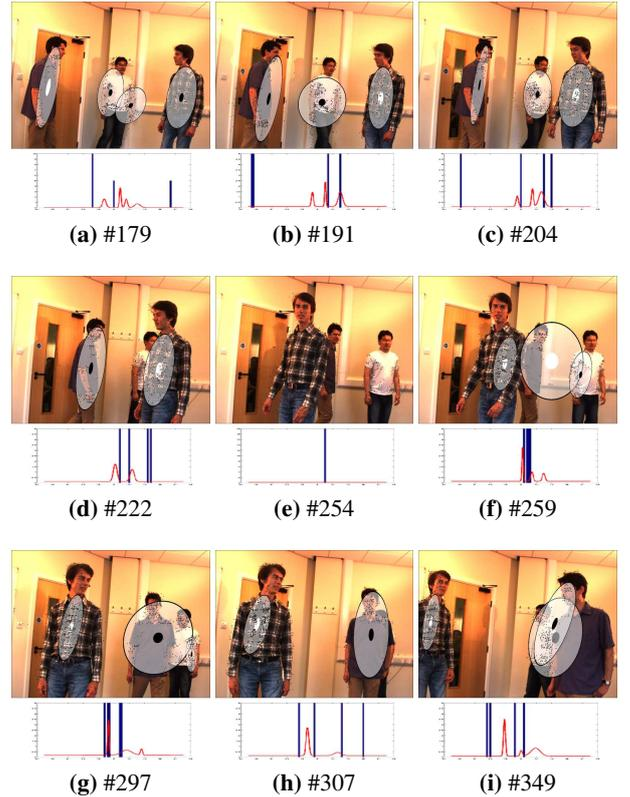
**Figure 3:** Results obtained with the CTMS3 sequence from the CAVA data set: Time intervals #179, . . . #349. The ellipses correspond to the 3D covariance matrices projected onto the image. The circle at each ellipse center illustrates the auditory activity: speaker emitting a sound (white) or being silent (black) during each time interval. The plot associated with each image shows the auditory observations as well as the fitted 1D mixture model.
