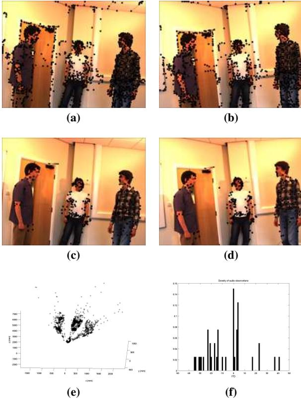
**Figure 2:** Interest points as detected in the left (a) and right (b) images. Dynamic interest points detected in the left (c) and the right (d) images. 3D visual observations within a time interval of  $\Delta T = 0.2s$ . (f) 1D auditory observations (ITD values) detected in the same time interval.
