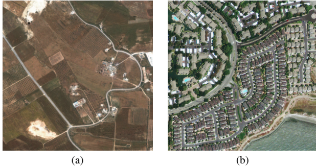
Fig. 1. Non-urban vs. urban remote sensing data for road extraction: (a) a 4 m resolution Ikonos image (Copyright ©Ikonos) of a countryside scene and (b) a Geoeye-1 image (Copyright ©GeoEye) of an urban area with 0.5 m resolution. Both images are 900 \times 900 pixel sized, for scale comparison.
