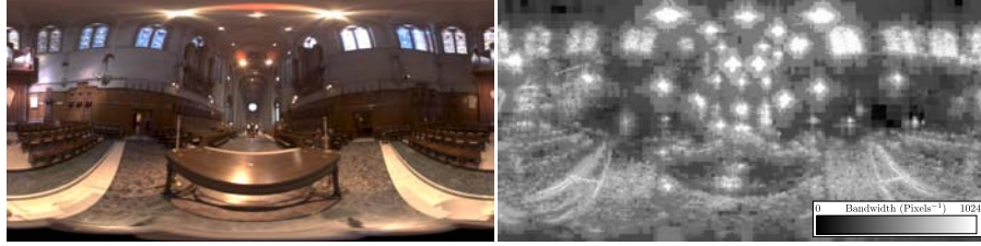
Figure 7: Right : Local angular bandwidth estimate for the environment map at left, computed from a 2D wavelet decomposition.
