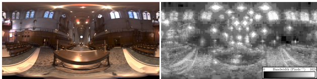
Figure 7: Right: Local angular bandwidth estimate for the environment map on left, computed from a 2D wavelet decomposition.
