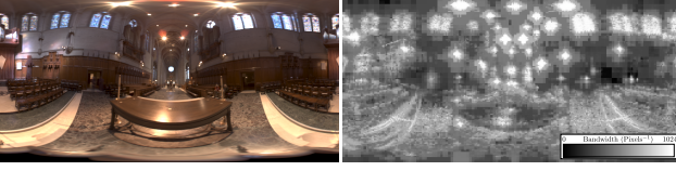
Figure 7: Right: Local angular bandwidth estimate for the environment map on left, computed from a 2D wavelet decomposition.
