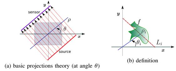
Figure 2. Radon transform.
