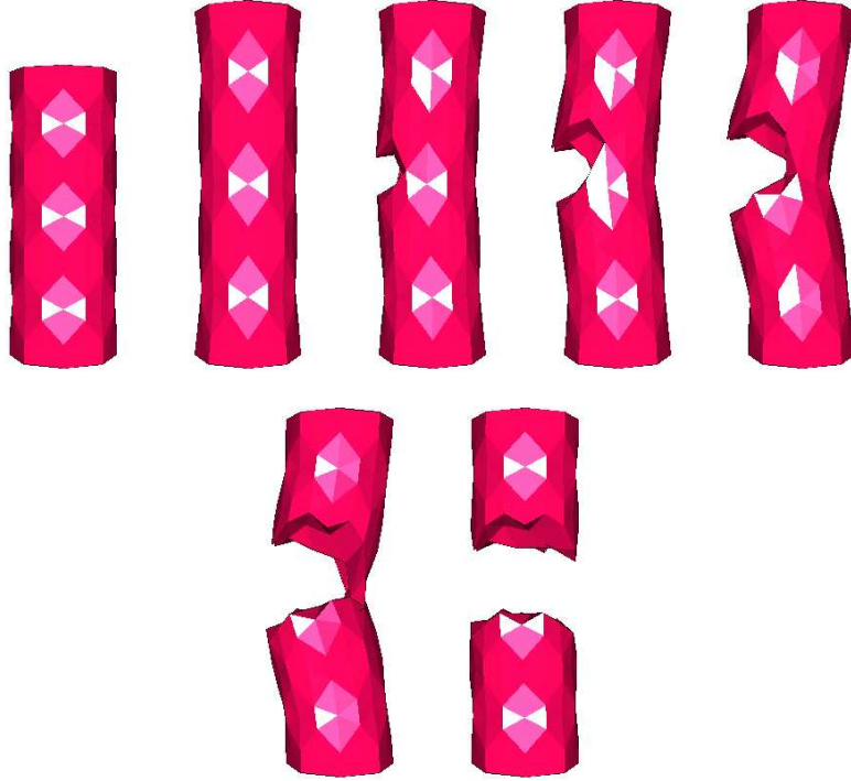
Figure 32: Deformation of a cylinder subject to gravity forces : some tetrahedra are progressively being removed at its center leading to a separation into independent solids.
