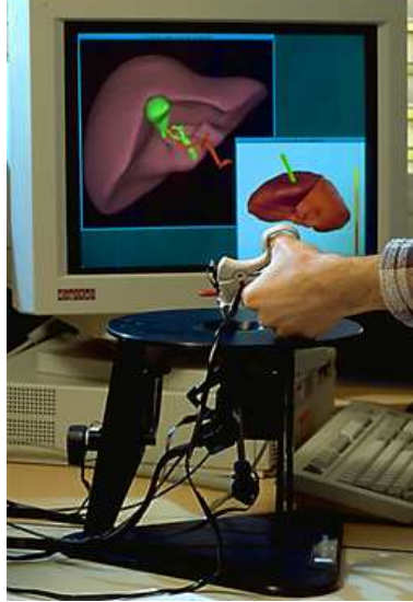
Figure 3: A force feedback system suited for surgery simulation
