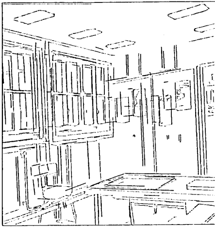
Fig. 20. Superimposition of 3-D segments of position 1 with 2-D edges of position 2 (crude initial motion estimate).
