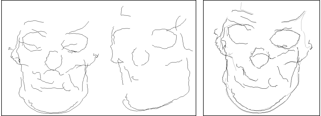
Figure 5: (a) Left: Crest lines on two 3D CT images of a skull obtained with the algorithm of Thirion and Gourdon. (b) Right: Superimposition of the lines of a. with our software in 7.7 seconds CPU on a DEC 5900. 8 curves are matched out of 15 and 32 curves. 53 points are matched out of 666 and 1124. Note that these experiments were performed before the DEC alpha architecture was available. CPU timings would be significantly decreased today.
