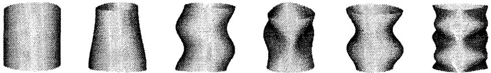
Figure 24 Energy-increasing vibration modes of a cylinder
