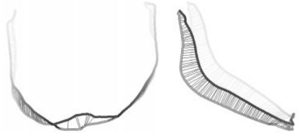
Figure 23. After interpolation of the missing correspondent points, we obtain the deformation D_i between L_i and L_i(\mathcal{C}) . We can check the result by applying D_i to L_i and comparing the obtained line (in black) with L_i(\mathcal{C}) which is displayed in the previous figure.
