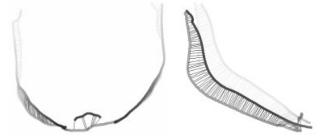
Figure 22. By using the registration algorithm, we can find the corresponding points between L_i (in grey) and L_i(\mathcal{C}) (in black). But some points of L_i remain without correspondent points because of the line topological constraints of the algorithm.
