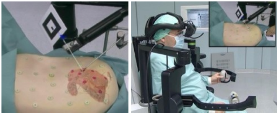
Fig. 8. By combining Augmented reality (left) and robotics (right) accuracy of image guided surgery may be improved and this may lead to additional levels of surgical automation (from [34]).
