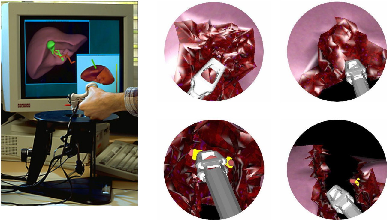
Fig. 4. (Left) A force feedback system suited for surgery simulation; (Right) View of the simulated hepatic resection involving linear-elastic materials (from [2], [64], [66] and [77], [62]).
