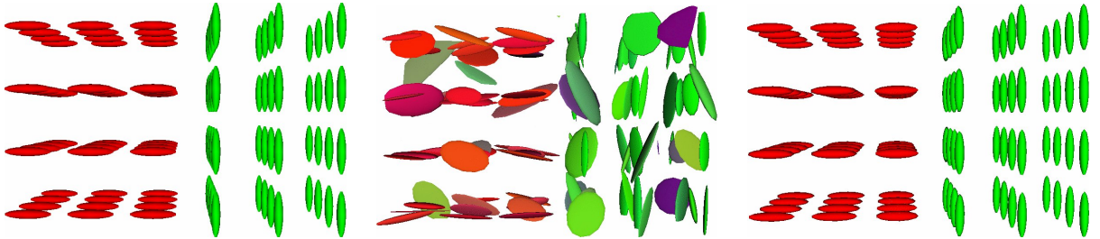
Figure 7: Left: 3D synthetic tensor field with a clear discontinuity. Middle: The field has been corrupted by a Gaussian noise (in the Riemannian sense). Right: result of the regularization after 30 iterations (time step \varepsilon = 0.01 ).
